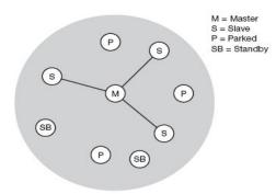
• If a parked device wants to communicate and there are already seven active slaves, one slave has to switch to park state to allow the parked device to switch to active state.
