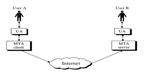
> SMTP also allows the use of Relays allowing other MTAs to relay the mail.
