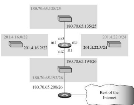
• Let us make a forwarding table for router R1 using the configuration as given in the figure above
