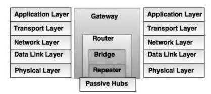
• Connecting devices are divided into five different categories on the basis of layers in which they operate in the network.
