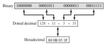
In *binary notation*, an IPv4 address is displayed as 32 bits. To make the address more readable, one or more spaces are usually inserted between bytes (8 bits).
