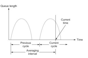
> Average queue length is measured over a time interval that includes the
